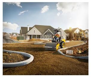
that is designed for commercial and residential site development, utility installations, driveways and landscaping jobs. Providing up to 12 degrees of oscillation and 41 degrees of frame articulation in each direction, the SD45B offers the stability and versatility required to compact in confined areas.
