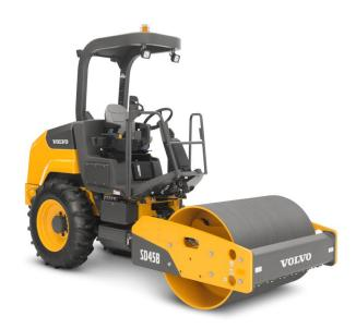
The Volvo Tier 4 Final D3.3 engine delivers high torque at low engine speeds, providing good fuel efficiency without compromising power. When controls are inactive for more than five seconds, the automatic idle feature reduces the engine speed, further decreasing fuel consumption. During the work process, the passive regeneration cleans the filters automatically without any input from the operator or negative impact on performance.
